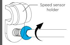
Now screw the speed sensor to the frame using the holder provided with a tightening torque of 0.8 Nm
