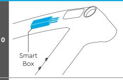
Smart Box installed and connected between the display and the wiring harness.
