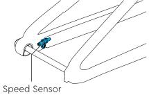
Speed sensor installed and connected to drive unit.
