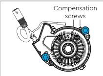
Adjust the two motor compensation screws to the correct frame width at the mounting points. Maximum axial frame tolerances of  $\pm$  1 mm can be compensated.
