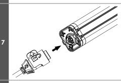
Connect the battery plug from the wiring harness to the battery.
