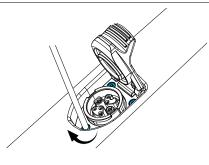
Position the charge port in the correct position in the frame using the charge port gripper (MTB) or by hand (Road).
