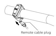
Insert the oval plug of the remote cable properly aligned and all the way into the remote control unit. Feed the cable within the handlebars in the direction of the display.
