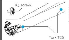
Fasten the Battery V01 to the frame with the TQ screws (M5) provided for this purpose and tighten them with a tightening torque of 3 Nm.
