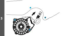
Insert the drive unit into the e-bike frame – matching the mounting points.
