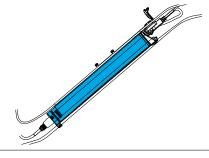
Battery installed in the frame and connected.
