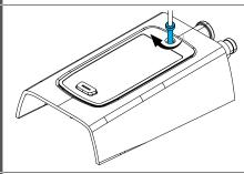
Tighten the included M3×20 display screw with a torque of 0.5 Nm.
