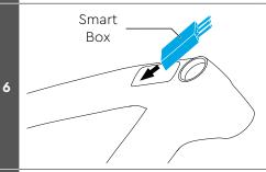
Insert the Smart Box into the display enclosure. To do so, first insert the cables into the display enclosure.
