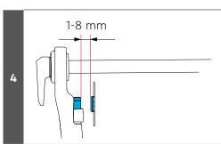
Check the air gap between the speed sensor and magnet. This must be 1-8 mm.
