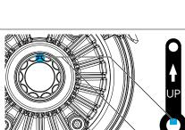
Mount both cranks, taking into account the index markings.
