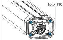
Screw the two brackets to the battery with the ISO14580 M3×6 screws (with threadlockers) with a torque of 1 Nm.
