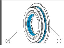
Prior to assembly of the lockring, grease the O ring ①
